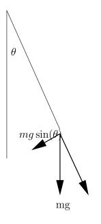
The pendulum bob makes an angle  $\theta$  with the vertical. The magnitude of the force (gravity) acting on the bob is mq.
